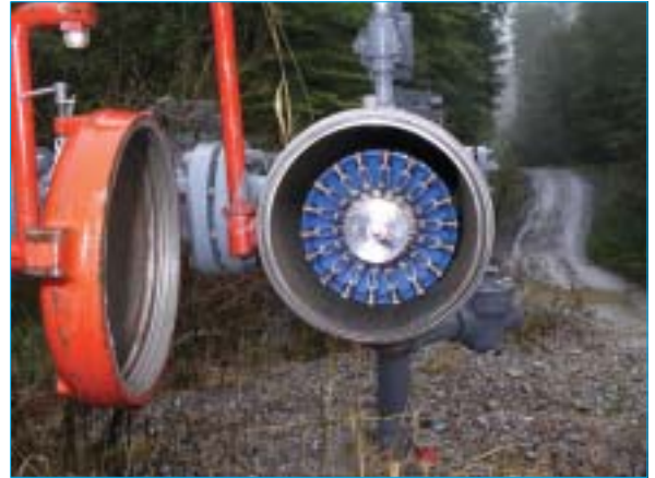
Weatherford's MultiCal™360 combined multi-channel caliper and SAAM smart utility pig.
