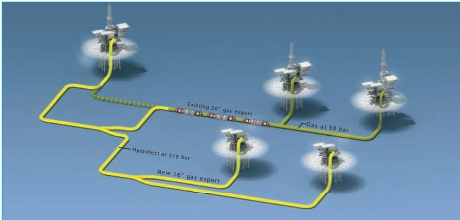
Layout of Shell's Shamrock and Caravel fields in the N Sea, and TDW's pipeline-isolation project.
