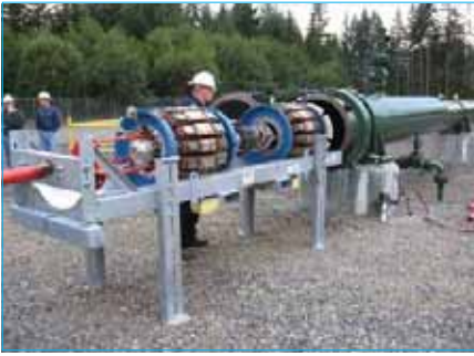
Fig.2. RoCD2 EMAT in-line inspection tool during the launch process.
