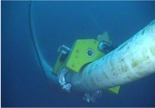
Customised MEC-Hug Crawler inspecting through the sag bend
