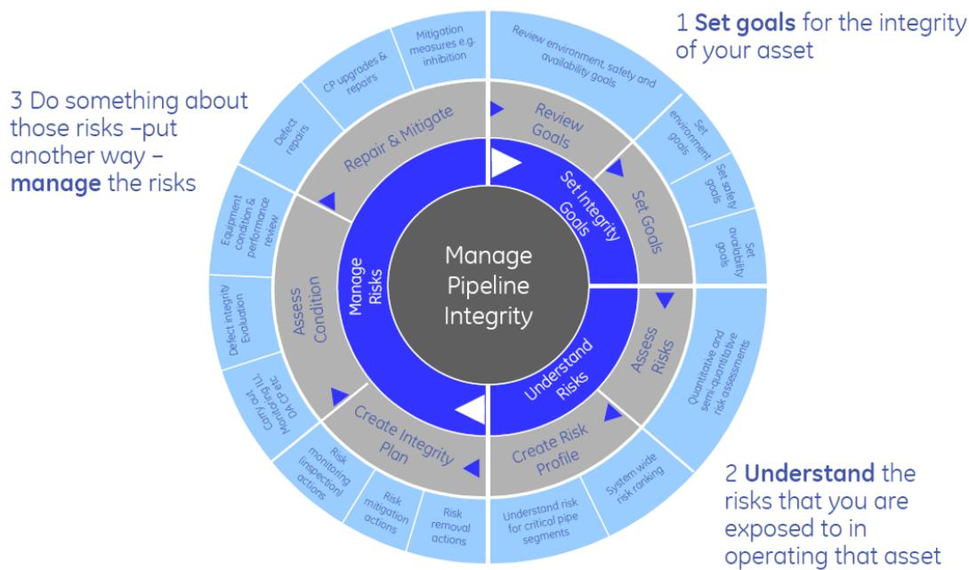
**Figure 2 – Pipeline Integrity Management Cycle**
