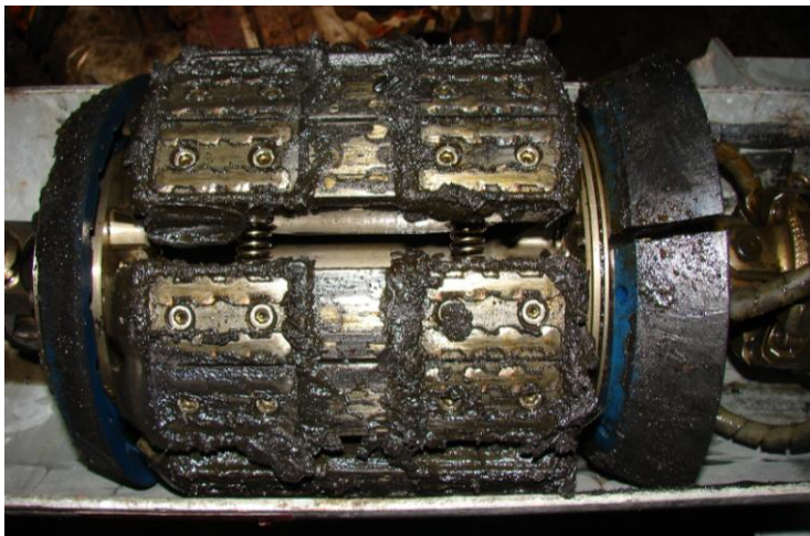
Figure 9: MFL tool after successful run in waxy pipeline
