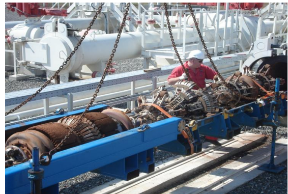
Figure 5: BSPC MFL Pig at Receive
