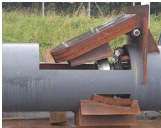
Figure 7: CATS Clapper Valve Test Rig
