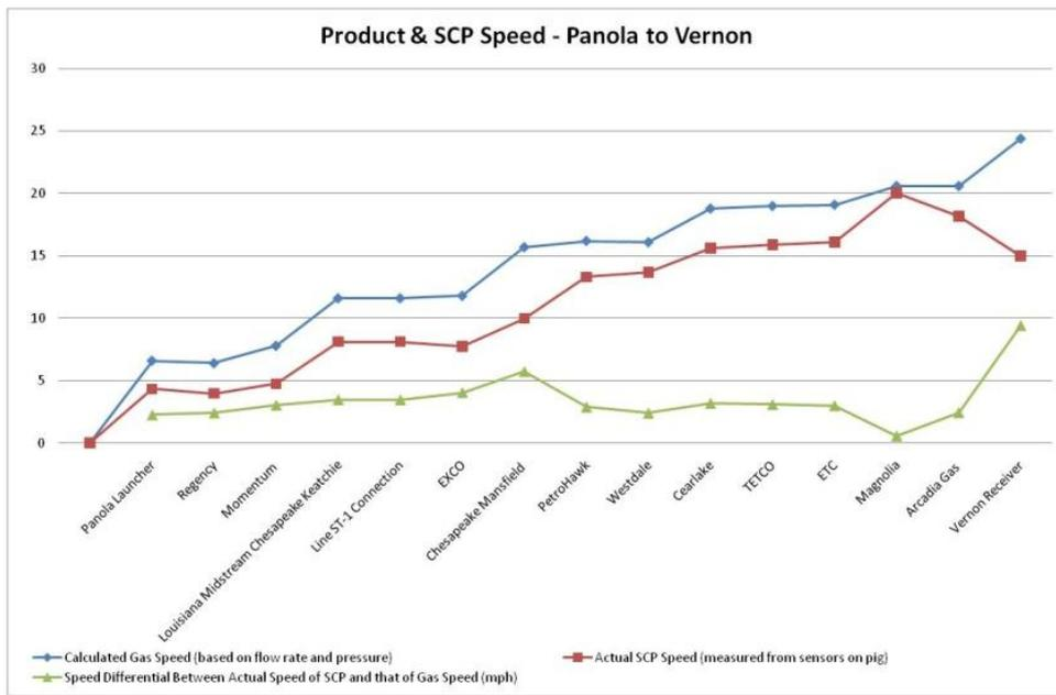
Figure 3.2: Gas and SCP speed
