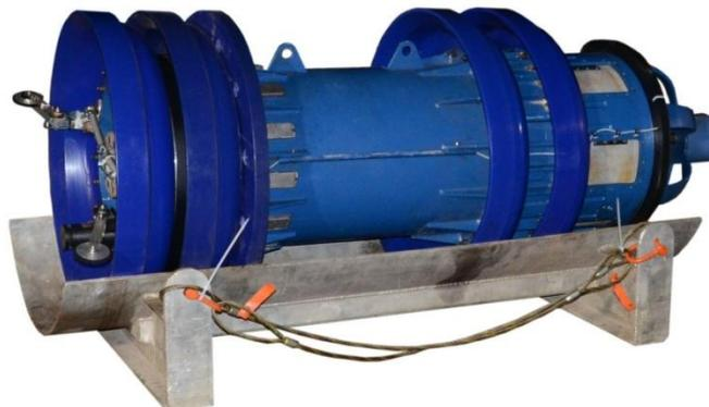
Figure 3.1: Initial 42" Speed Control Pig
