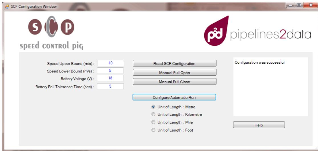
Figure 2.4: Configuration of the SCP in software
