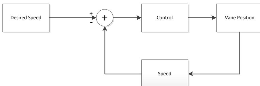
**Figure 2.3: Closed loop control system**
