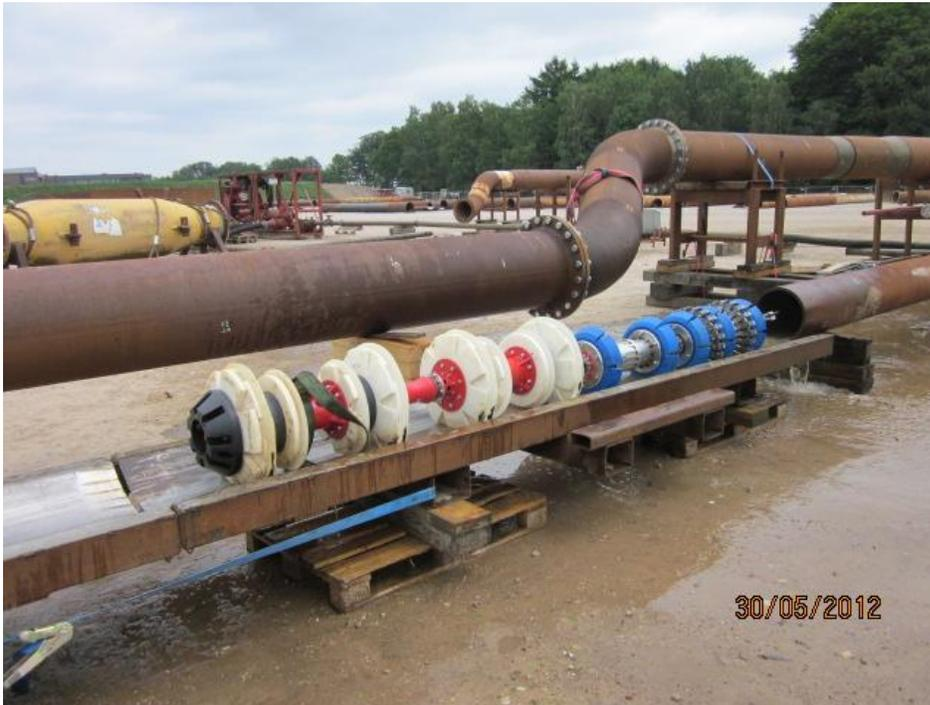
**Figure 6: The RoCorr-SIC ILI tool during testing at the ROSEN Technology and Research Centre.**
