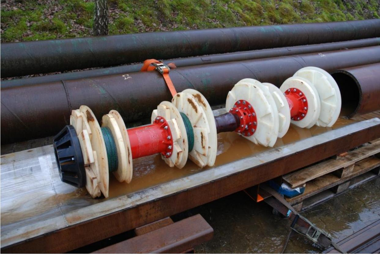
**Figure 3: ROSEN pig configuration at test facility**
