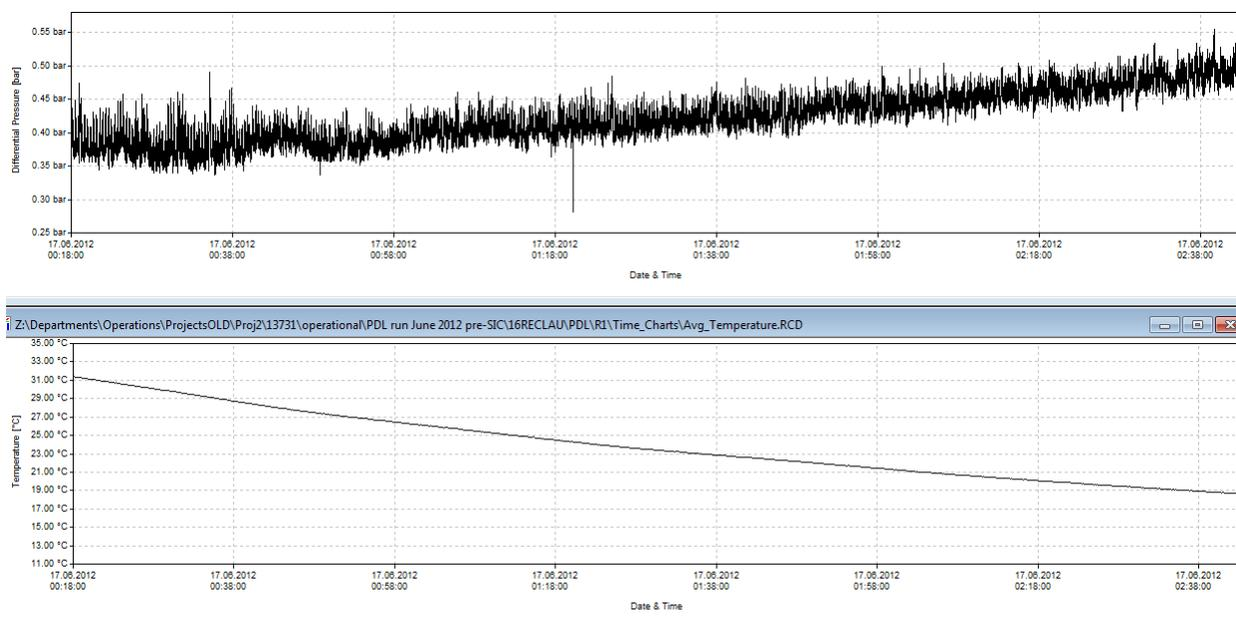
**Figure 5: Gradual rise of differential pressure (top) due to wax deposition at decreasing temperature (bottom).**
