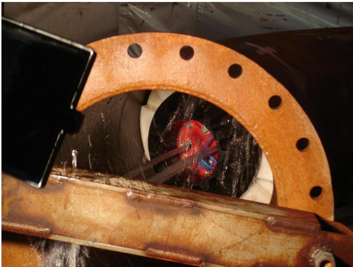
**Figure 4: Bypass of water through open nozzles during testing in 20" bend.**
