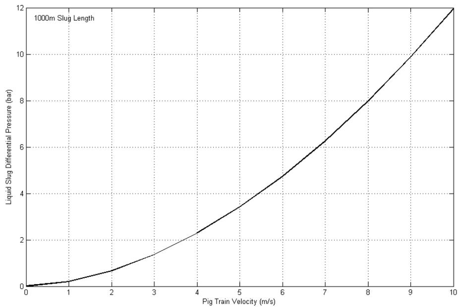
Figure 10, Output for 20" Gas Pipeline pig train velocity profile
