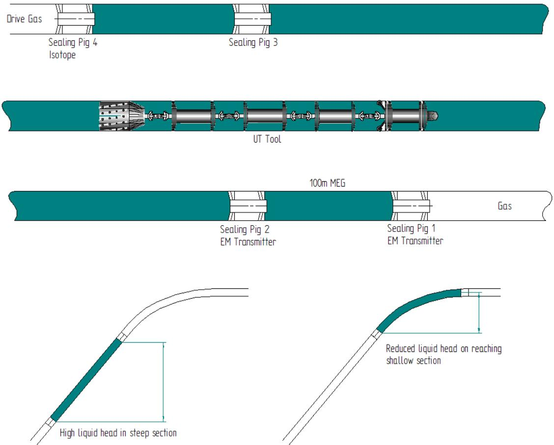
The effect of the reduction in liquid head is to accelerate the train
