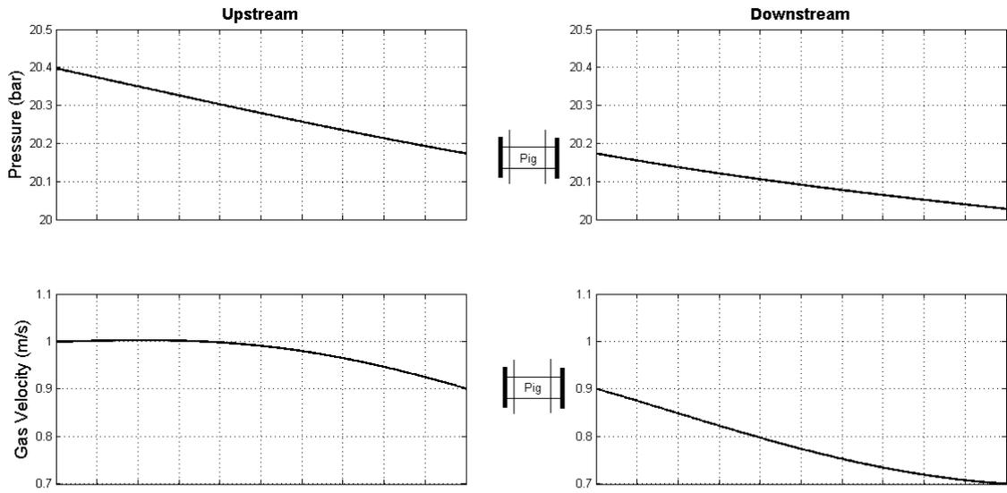
Figure 4, Effect of pressure on the motion of a pig
