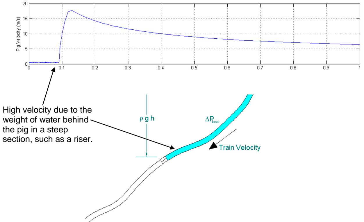
High velocity due to the weight of water behind the pig in a steep section, such as a riser.
