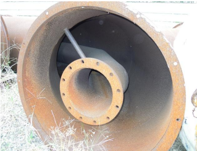
Figure 2: Photo of the Mitre bends inside the pipe in pipe configuration
