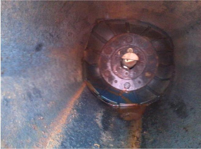
**Figure 9: Bi-di Pig Stuck in Restriction**
