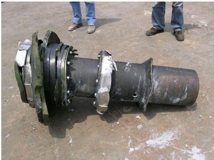
**Figure 1: Gauging Pig After Recovery from Sea Line 2**
