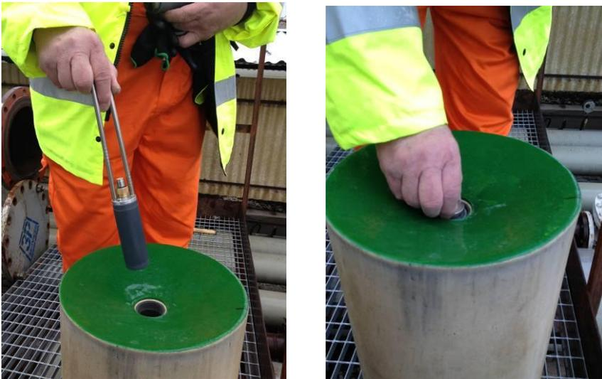
**Figure 4: Loading Caliper Module and Transmitter**
