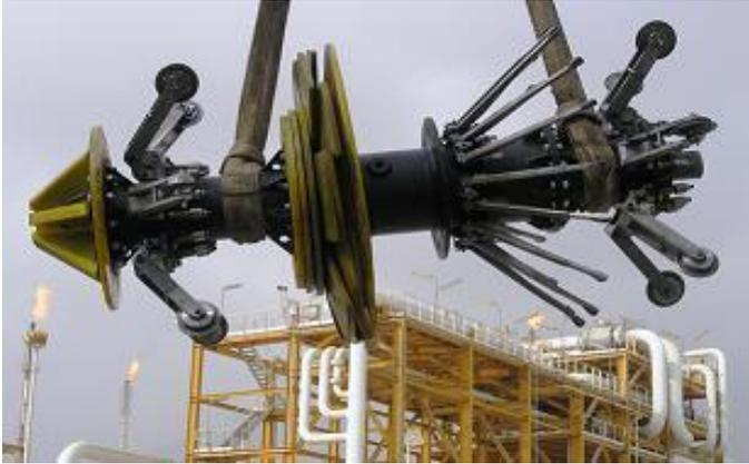
**Figure 2: Caliper Pig After Recovery from Sea Line 2**
