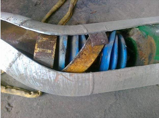
**Figure 3: Bi-Di Pig With Dislodged Anodes**
