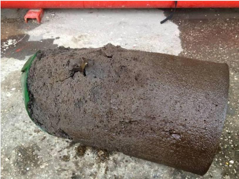
**Figure 5: Anode Retaining Strap Embedded in Pathfinder Pig Body**
