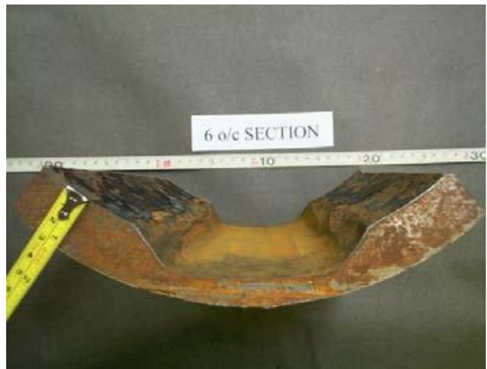
**Figure 2: Groove Corrosion on the Strathspey Water Injection Pipeline**
