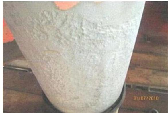
**Figure 4: External Corrosion Area above Neoprene Splash Zone Coating**
