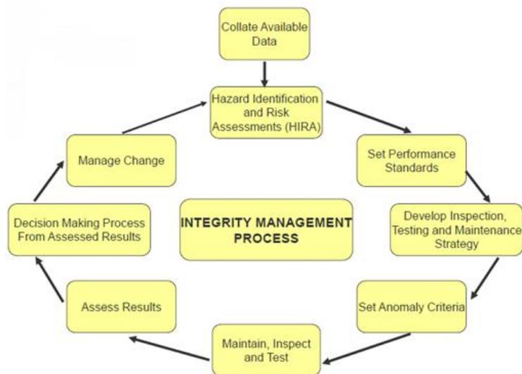
Figure 1: CNSL's Integrity Management Process
