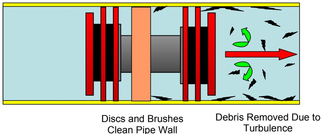
The turbulence within the fluid flow will hold any small, solid debris in suspension, effectively sweeping it out of the line. The use of bypass ports through the pig can aid this sweeping effect.
