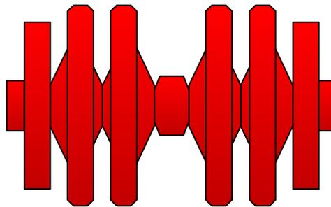
Both sealing and guide elements are cast as a single component in polyurethane.
