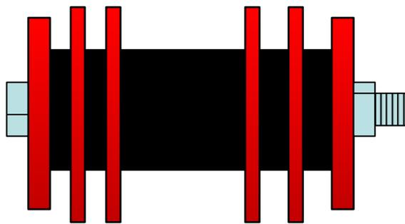
Similar to the mandrel pig, the elements are fitted to a single bolt, rather than a solid body.
