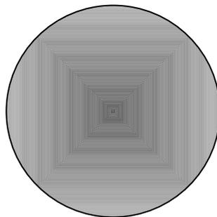
Spheres can be solid or inflatable with air, water, or glycol and are used for product separation, liquid removal, and in meter proving.
