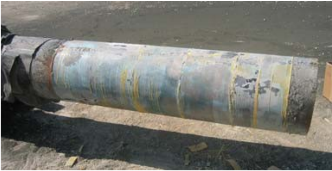
Figure 8 - Section of Clock Spring Removed by Sandblast
