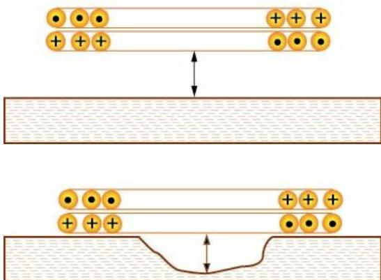
Figure 3. Liftoff distance measured by eddy current coil pair.
