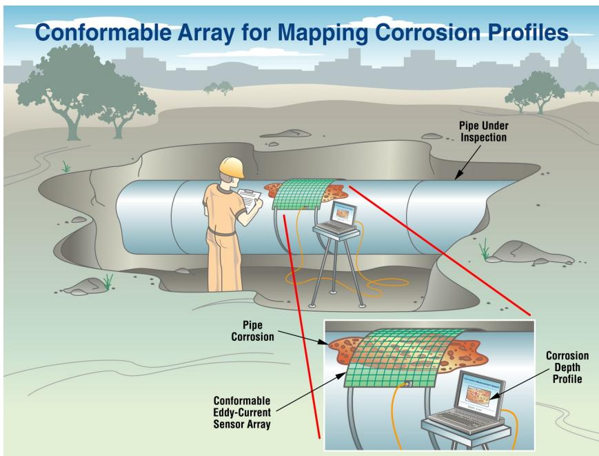
Figure 4. Flexible array concept
