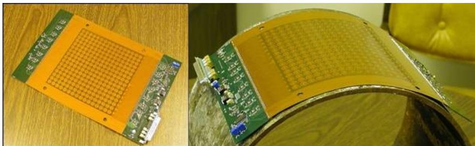
Figure 5. Conformable EC Array
