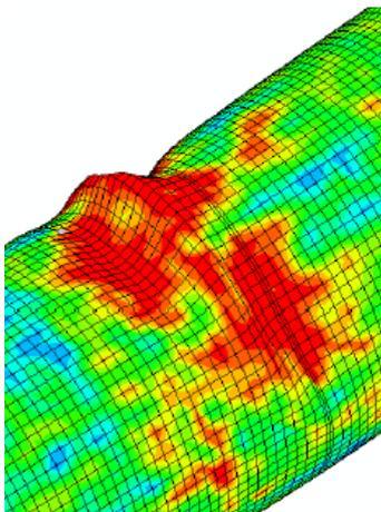
Figure 6 – Results of Environmental Loading of a Buckle
