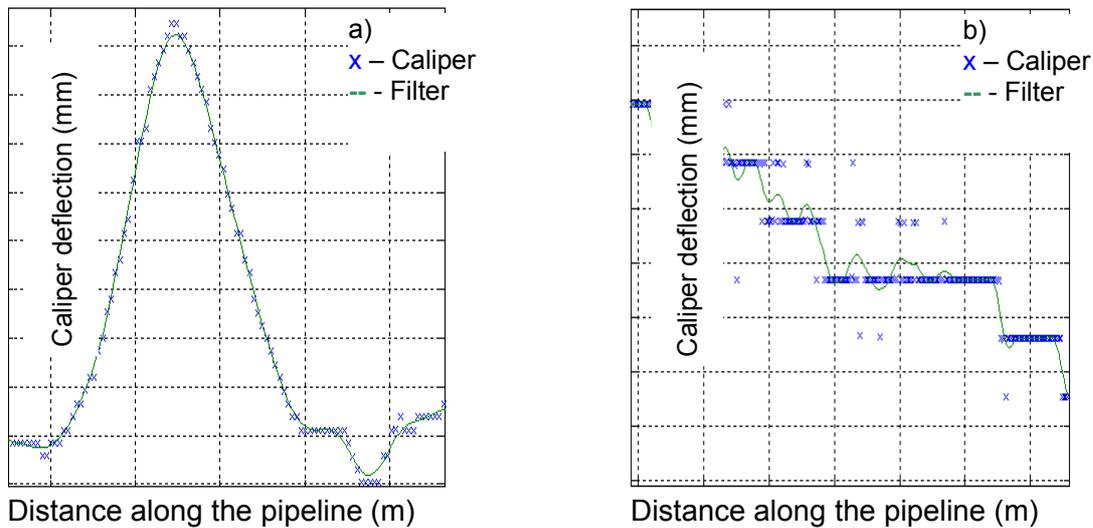
Figure 4 – Geometric Data Filtering and Fitting, Using a Narrow Window.
