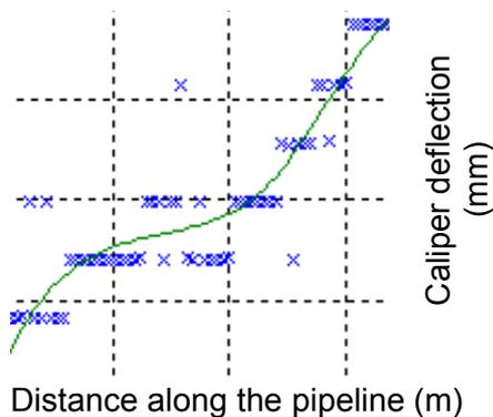
Figure 1– Example of a Caliper measurement, demonstrating significant quantization of signal and noise.
