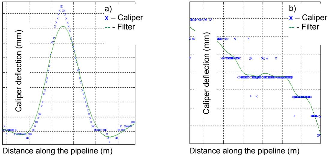
Figure 3 – Geometric Data Filtering and Fitting, Using a Wide Window.
