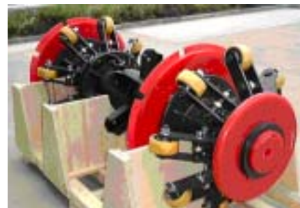
Fig.3. Pipeline cleaning pig, before...
