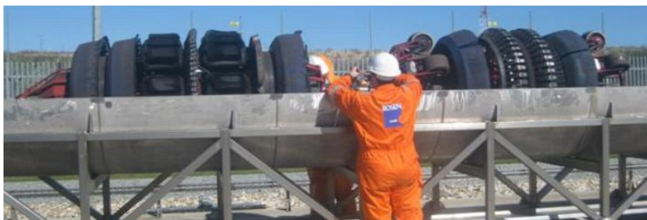
The customized RoCorr-MFL/SIC in-line inspection tool has arrived in Easington, England after a historic non-stop run through Langede Pipeline
