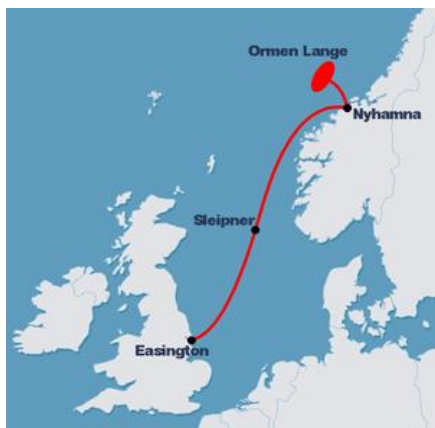
Route of Langede Pipeline, the world's longest subsea gas pipeline
