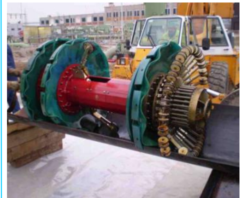
PSI's Multi-channel inspection tool
