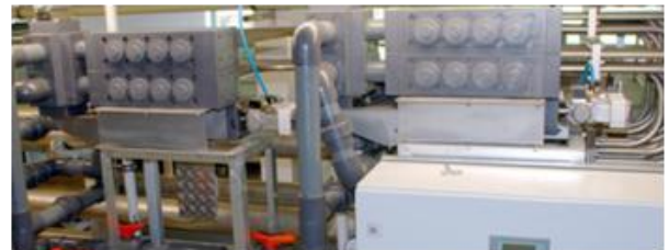
Fig.: 2 pig stations (dark grey boxes), each station controls 4 pigs in 4 different pipelines
