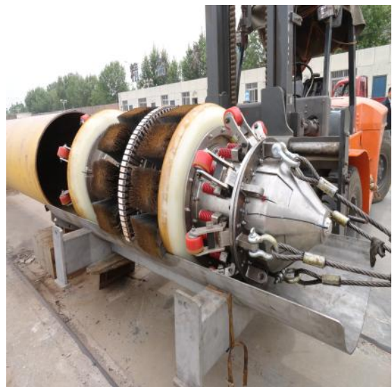
CPPI launches 40" and 48" Tri-axial MFL inspection tool ●
