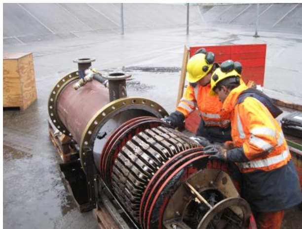
A 30" Bi-directional tool with temporary pipe spool upon completion of 1 st inspection run
