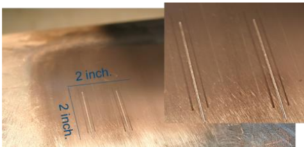
Surface grooves from two HSD Tests on pipe exterior surface
