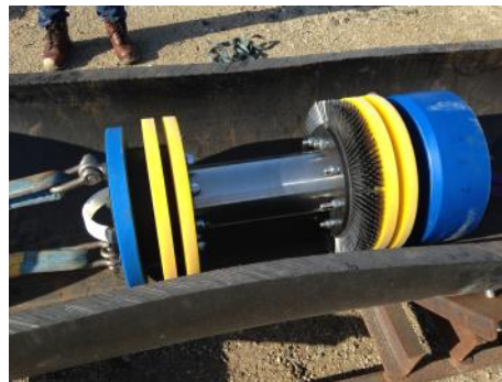
A 16" Pioneer Smart Utility Pig ready for pull tests at PRCI TDC
