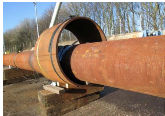
Pull-through line build with simulated caisson and pipe defects at 6 o'clock position
