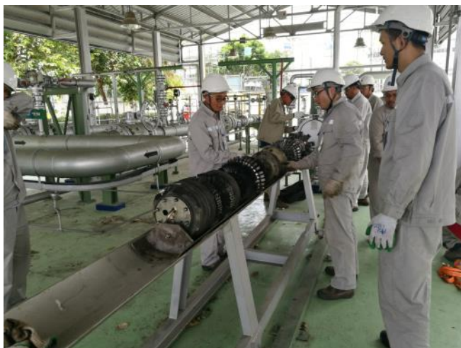
CPPI's triaxial magnetic flux leakage (MFL) inspection tool. ●
