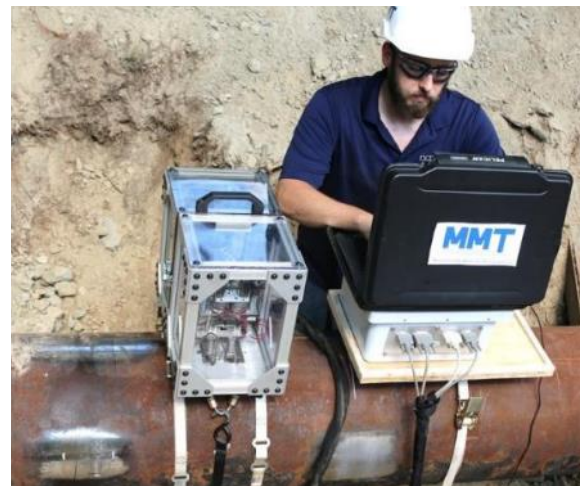
HSD Tester attached to a pipeline in the field
