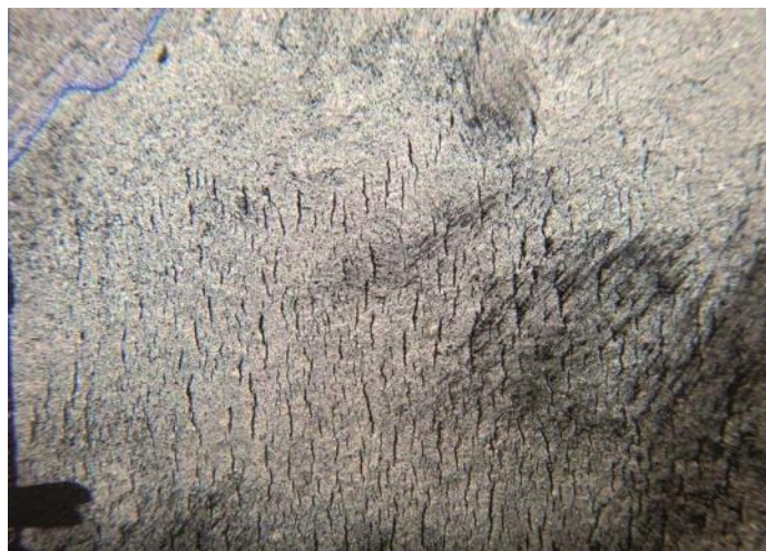
Circumferential crack field detected with ILI results using UCc
