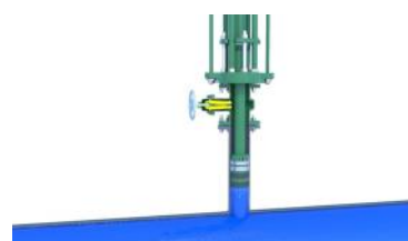
Hot Tap Clamp and BISEP Removed, New flange and Valve Installed
