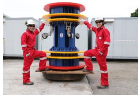
Dacon's 52" UT-R Pig Inspection
