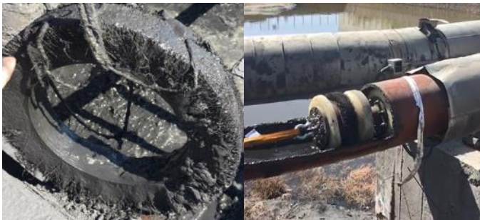
Steel Brush Cleaning Pig pull through test & Slurry Soaking test on steel brush
