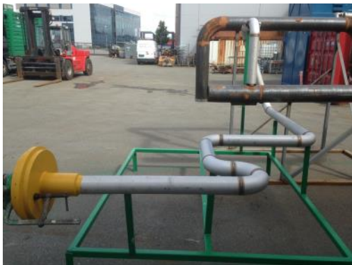
Figure 1 – Mock-up of the manifold.
