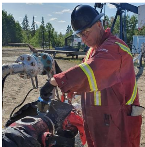
Pioneer tool being dropped into a typical pig valve
