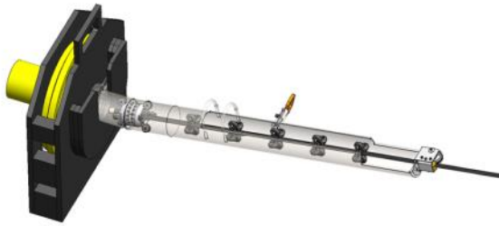
Figure 3 – Black protection cap and “snap-on” launcher arrangement.
