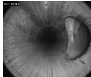
Figure 4: Verification of an unbarred tee
