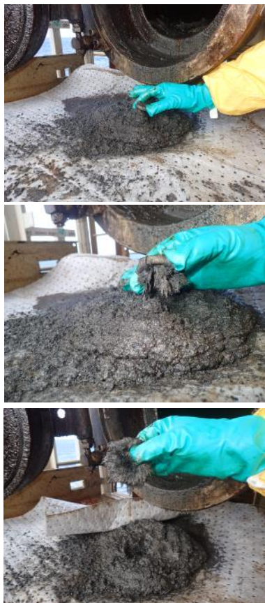
Ferromagnetic debris taken out by the HMCT
