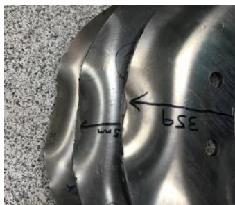
Figure 2: Gauge plates with unexplainable deformation
