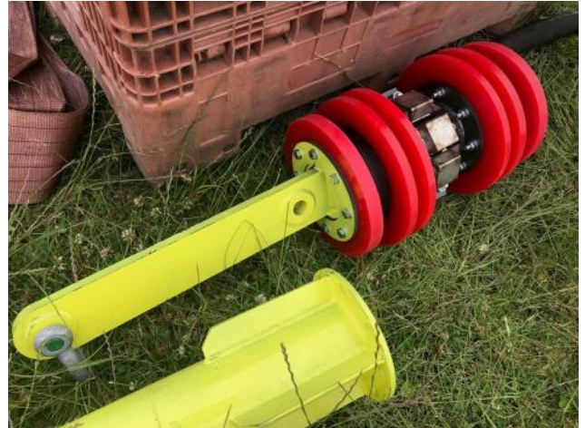
12”NS Cable pull through pig
