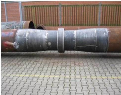
View of 30" gate valve in 34" pipe simulation
