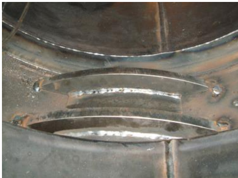
Simulation of partially closed valve
