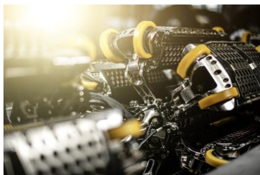
Next generation ILI technology featuring a state-of-the-art Phased Array inspection system
