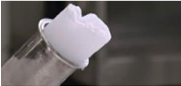
Figure 2. showcases how the ice slurry is formed into a solid know as an “ice-pig” once pumped into the pipeline.
