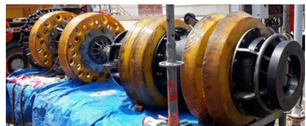
Speed Control Unit (front body - right) and GEO Tool (rear axle - left) before the run
