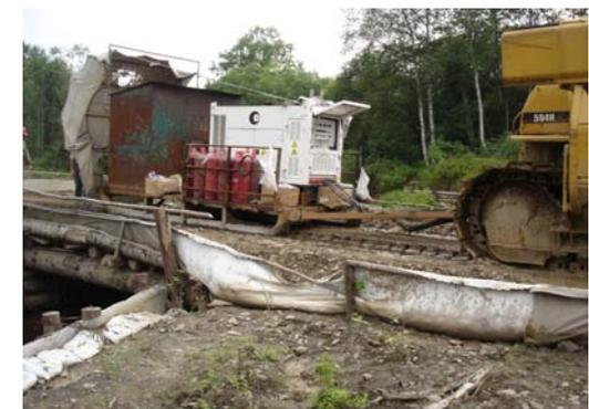
Figure 16: Tracked vehicle pulling equipment “sled” to site through the mud
