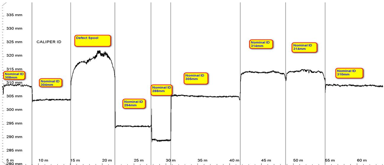
**Figure 10 Comparison of Internal Diameter**
