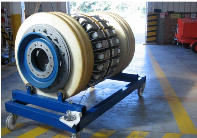
Fig. 5: Single module 42" MFL inspection tool
