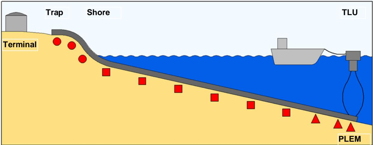
Fig. 1: General layout of the Ocesa tanker loading system and 3P Services' antennae and markers
