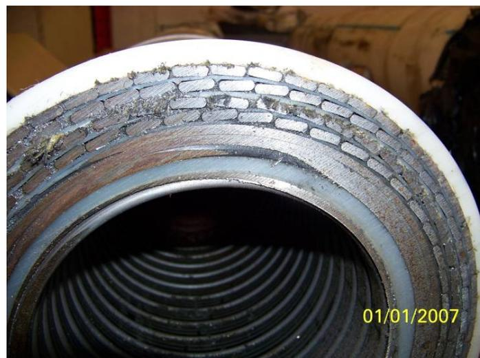
**Figure 5: Typical appearance of a flexible pipe**
