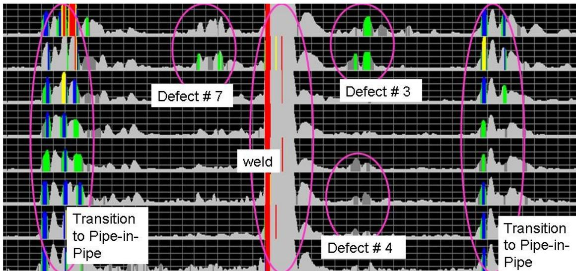
**Figure 4: Detected eddy current signals in clad pipe**
