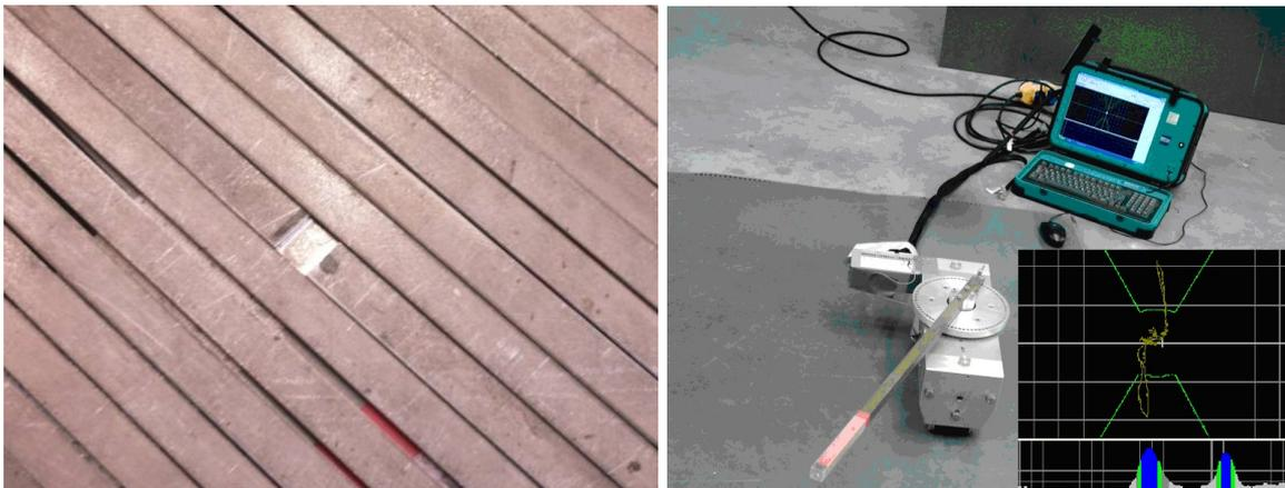
**Figure 7: Testing and calibration for certain defect types and sizes can be done on a flat sample.**
