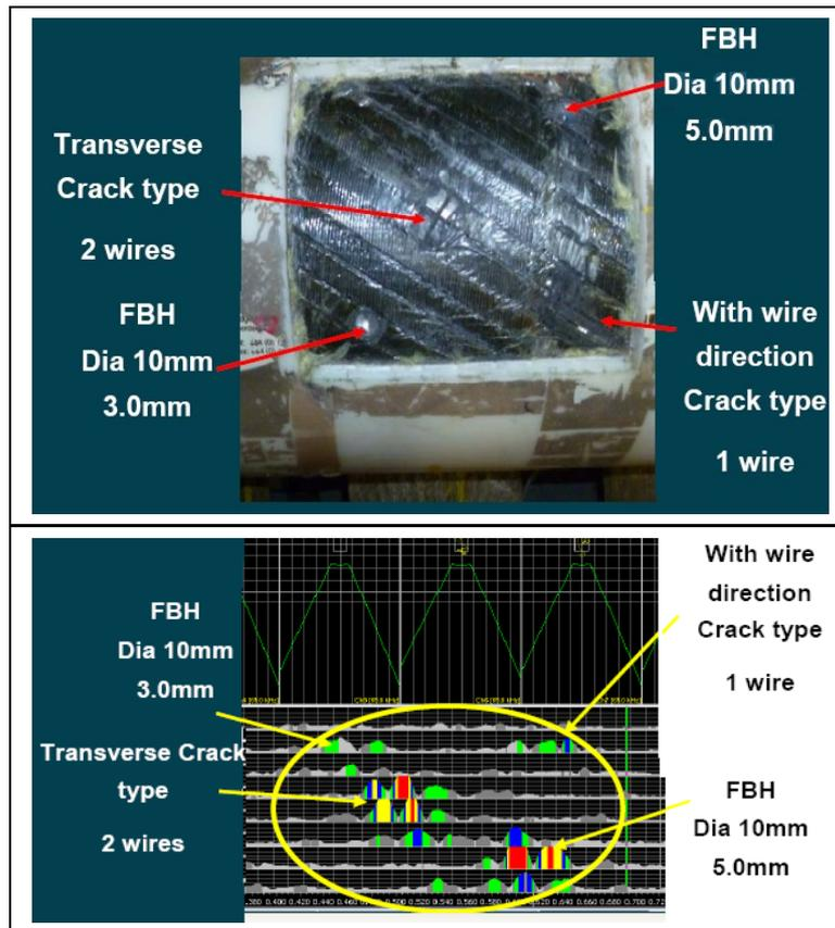
**Figure 8: Upper part: artificial defects in a flexible riser pipe; Lower part: The signal obtained from defects in a flexible riser pipe.**
