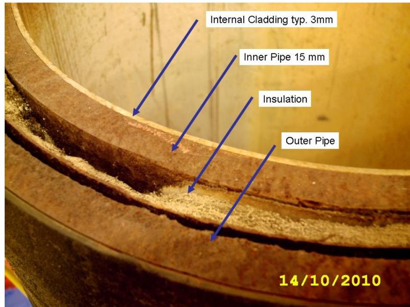
**Figure 2: The cladded pipe consists of an inner CRA layer. In this particular pipe there is also an outer ferritic layer. Test defects were in the inner ferritic pipe.**
