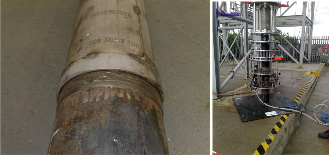
**Figure 1: Monel cladded pipe on the left and an external inspection device made by Innospection**
