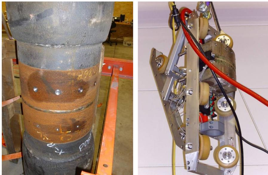
**Figure 3: Test set-up with external defects in a cladded pipe and inspection device used for the test**
