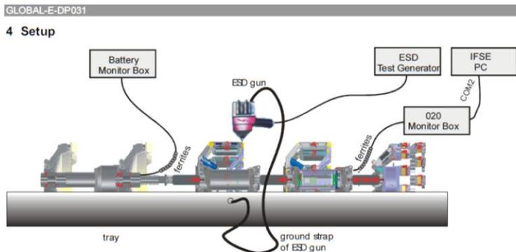
Fig. 1: Example for an entire test setup (SmartScan 207/26)
