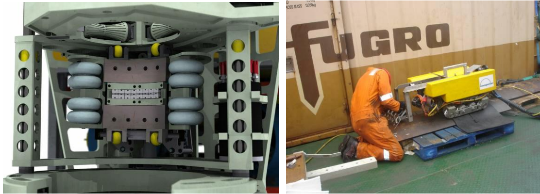
Figure 9: Left: The scanner inside the frame of the MEC-FIT unit. Right: A different sub-sea scanner unit is equipped with nozzles for a prior cleaning operation
