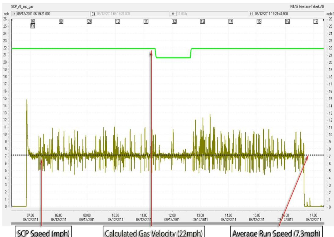
**Figure 3.5: Gas Speed Velocity, SCP Speed**
