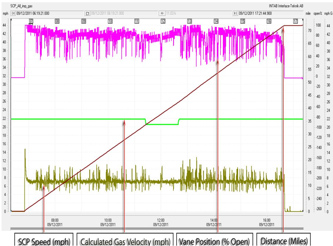
**Figure 3.6: SCP Speed, Calculated gas flow velocity, Vane position and Distance**
