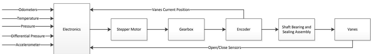
**Figure 2.1: System Block Diagram**
