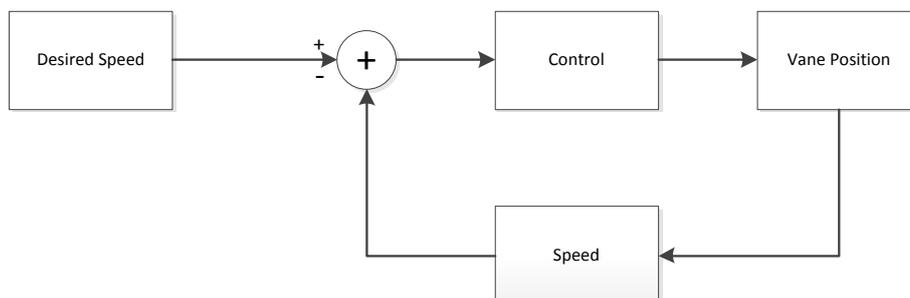
**Figure 2.3: Closed loop control system**
