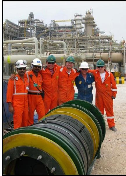
**Figure 7: 38" Tecno Plug™ after Sour Gas Deployment**
