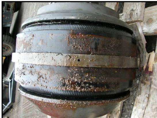
**Figure 12: BISEP™ Head after Successful Set on Hot Tap Swarf**
