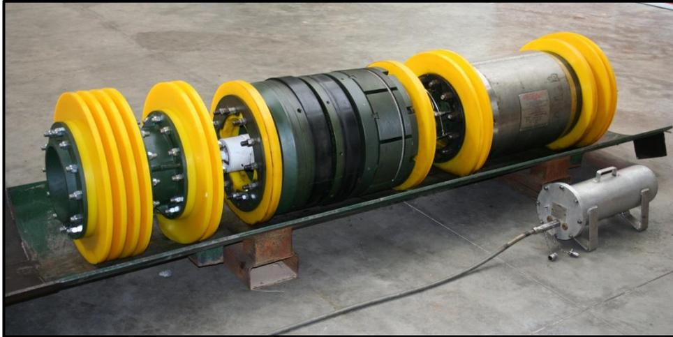
**Figure 5: Remote Control Tecno Plug™ in Pigging Configuration**
