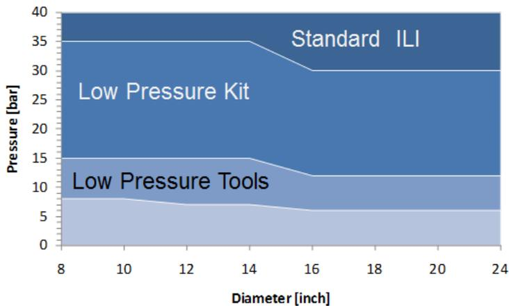
Figure 12: Tool selection guideline for low pressure gas pipelines
