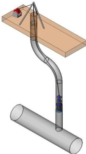
**Figure 3: Schematic illustration of gravity based/pump in – pull out approach**
