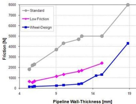
Figure 10: Dynamic friction force demonstrated for different cup designs
