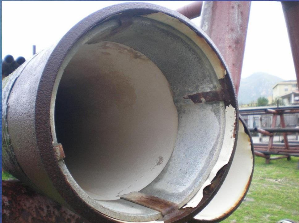
Internal Anodes On Similar Pipeline
