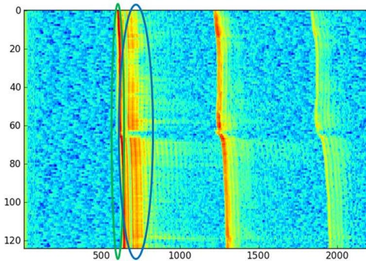
**Figure 27: UT data for 6in pipe spool**
