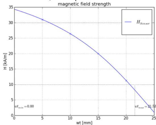
Figure 13: magnetic field strength vs. wall thickness
