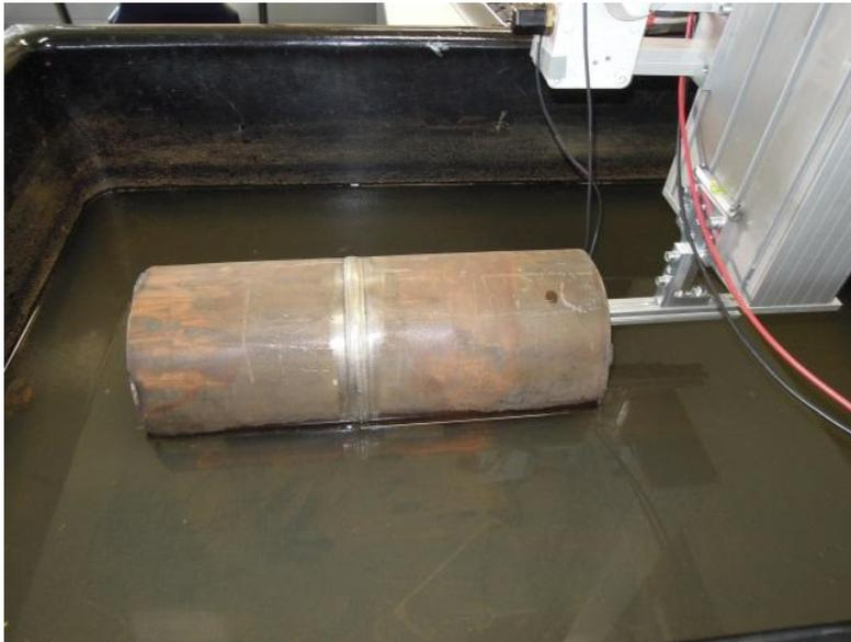
Figure 26: Test setup for test with ultrasonic sensors
