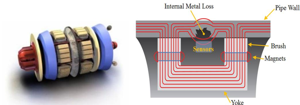
**Figure 7: RoCorr MFL-A Tool and flux line distribution**
