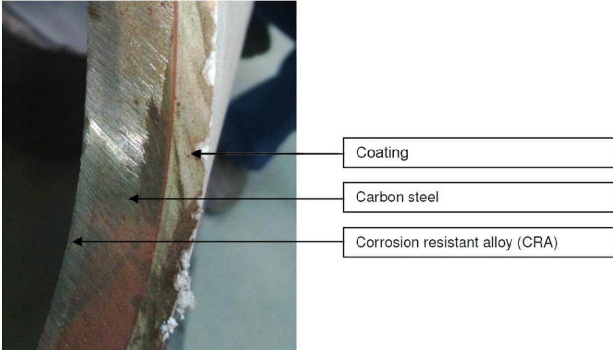
**Figure 4: CRA pipe showing carbon steel and CRA layer**
