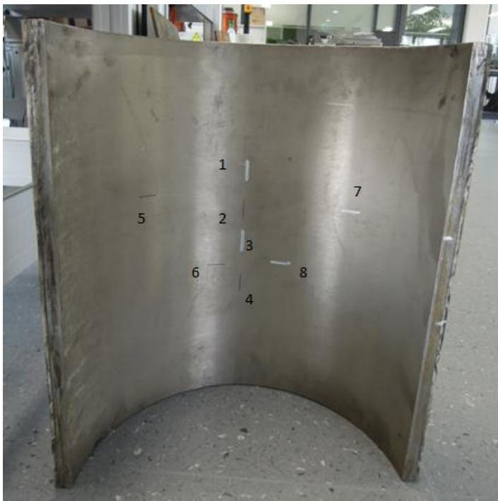
**Figure 30: UT crack detection test setup with 16in pipe spool**
