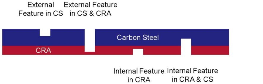
**Figure 8: Schematic picture of types of features**
