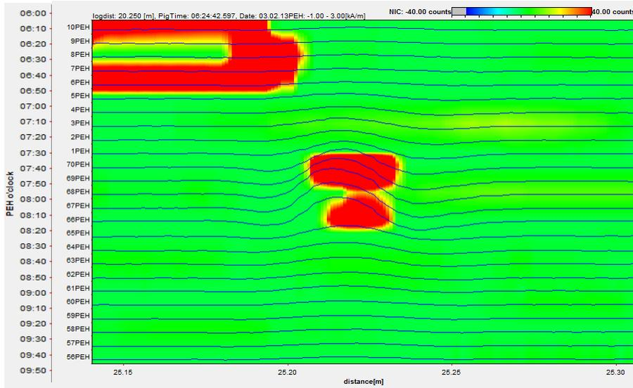
Figure 12: MFL data plot of feature four
