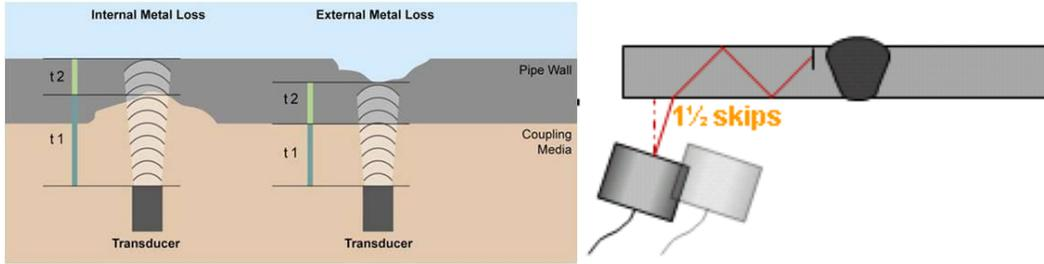
**Figure 21: Ultrasonic principle (left metal loss, right crack detection)**
