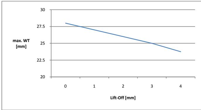
**Figure 14: maximum wall thickness vs. lift-off**
