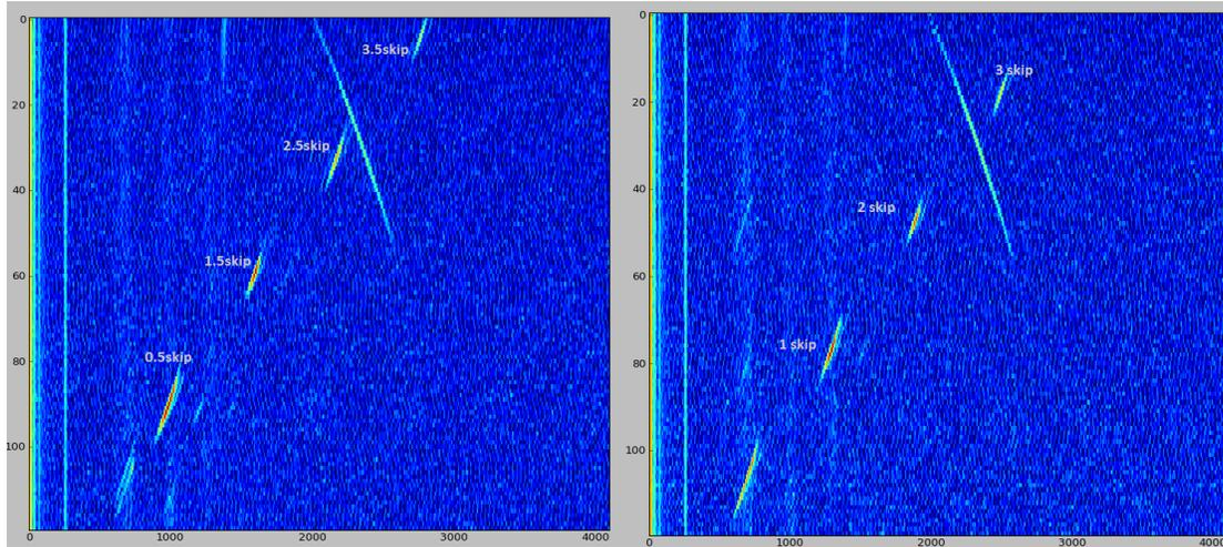
**Figure 31: UT crack detection data for 16in pipe spool (left external, right internal)**
