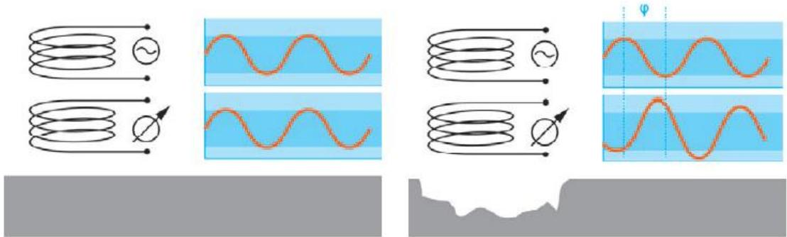
**Figure 16: Principle of eddy current**
