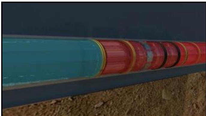
The first plug is then fully set (seals compressed onto pipe wall).
