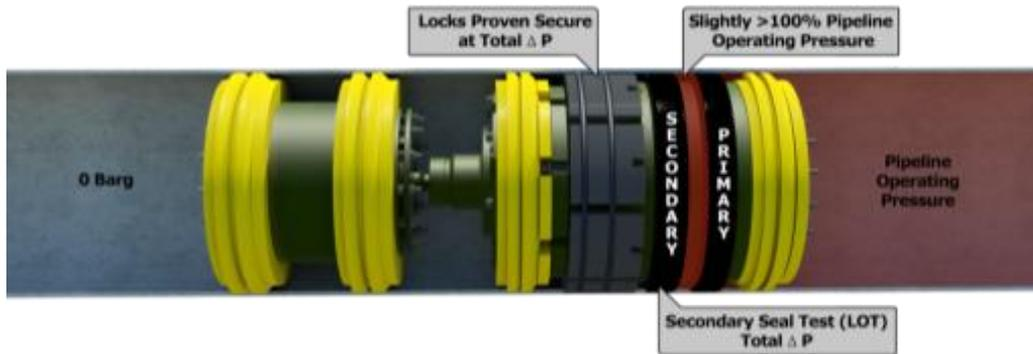
Figure 14: Secondary Seal Test
