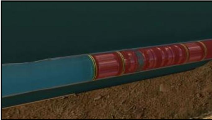
Before reaching the line defect the plug is partially set (locks only) and the through port vent opened.
