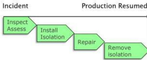
**Figure 5: Emergency Pipeline Repair Timeline – With Isolation Tools**
