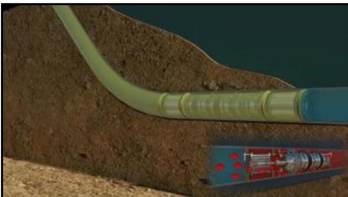
As the second plug is pigged, the product between the plugs passes through the partially set first plug.
