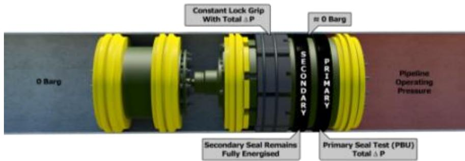
Figure 15: Primary Seal Test
