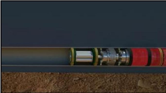
Pressure between the seals is monitored to prove the Secondary seal.
