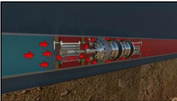
Opening the through port allows the second plug to be pigged from the other end of the pipeline - towards the first (partially set) plug.
