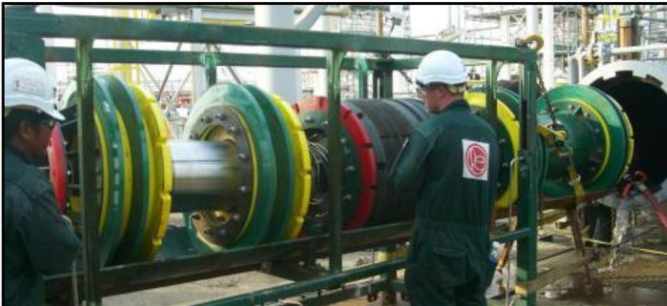
Figure 12: 36" Remote Tecno Plug™ Deployment Malaysia
