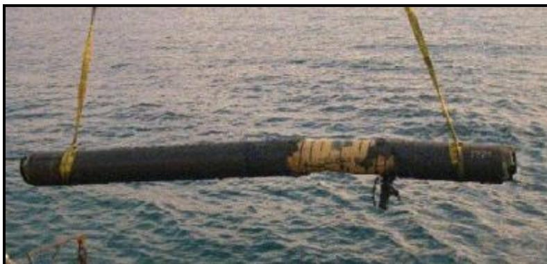
**Figure 2: Cut Out Damaged Section of Pipeline**
