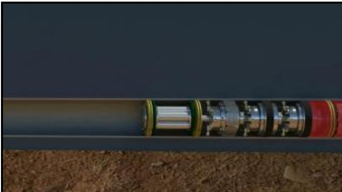
The annulus between the seals is vented to produce a zero energy zone.
