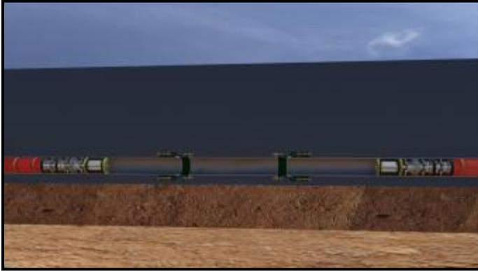
New section of pipe installed using mechanical connectors or hyperbaric weld.
