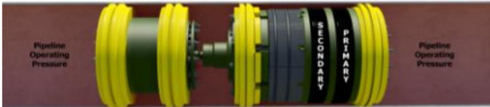
Figure 13: Pressure Equalised on both sides of Plug
