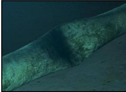
**Figure 1: Unpiggable Defect in Pipeline**
