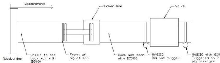
By being able to profile the debris in front of the pig and the clear line behind the pig, OEL was able to indicate the exact pig location with three confirmations that the pig had entered the receiver and was stuck 4.1m from the receiver door at the kicker line. At this point operators had all the information necessary to open the receiver door, clear out the debris and retrieve the pig.
