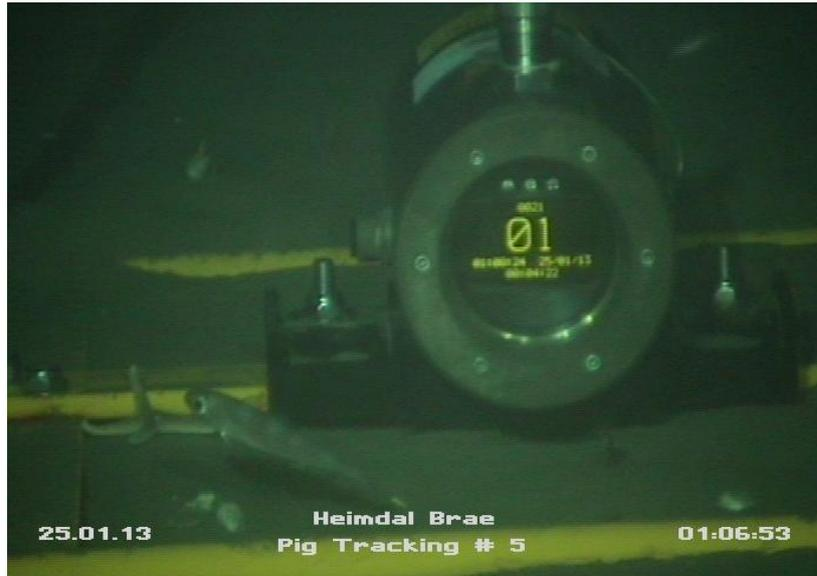
**4000SD Unit above Buried Line at Heimdal to Brae Pipeline (Detected Pig Passage)**
