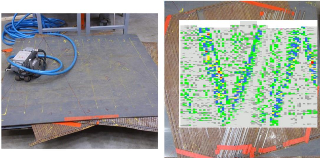
**Figure 8: Set-up for testing of wire disorganization defects on a flat sample (left) and results for loose wires and wire gaps (right).**
