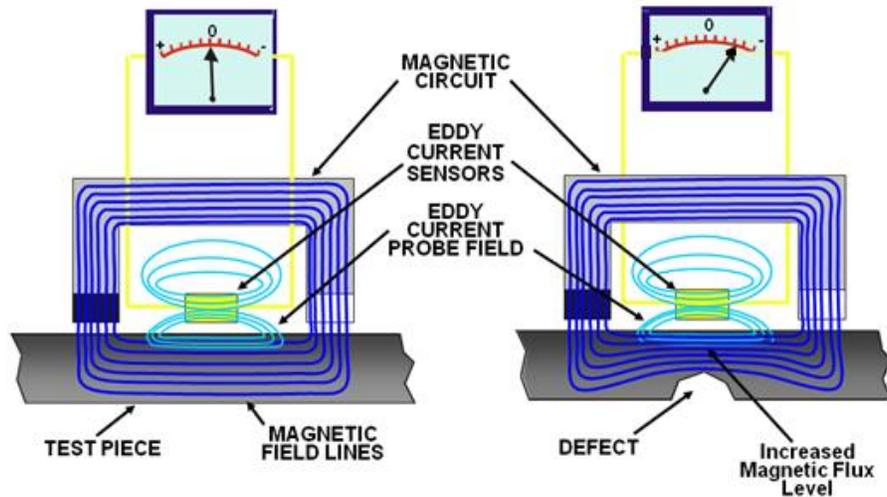
**Figure 2: Principle of the MEC technology (Magnetic Eddy Current) also known as a further developed technique from Saturation Low Frequency Eddy Current (SLOFEC).**
