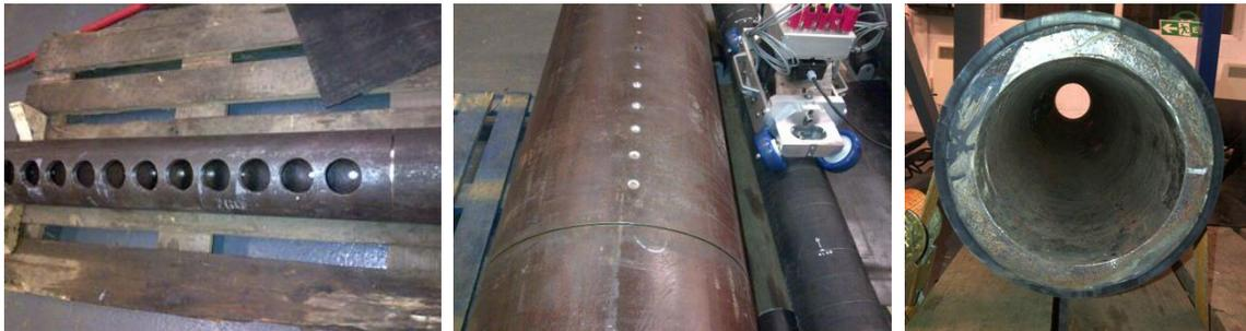
**Figure 4: Test pipe for the riser inspection with artificial defects. Internal defects were introduced through a hole on the opposite side.**
