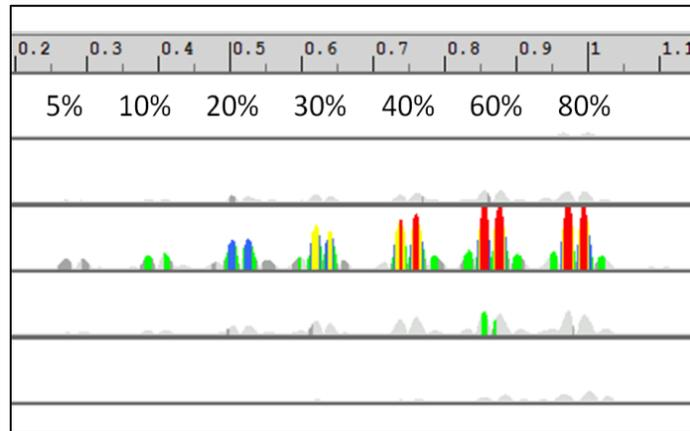
**Figure 7: Sequence of 20 mm near-side defects in an 8" pipe of 23 mm wall thickness under 12.7 mm ( $\frac{1}{2}$ " ) coating.**
