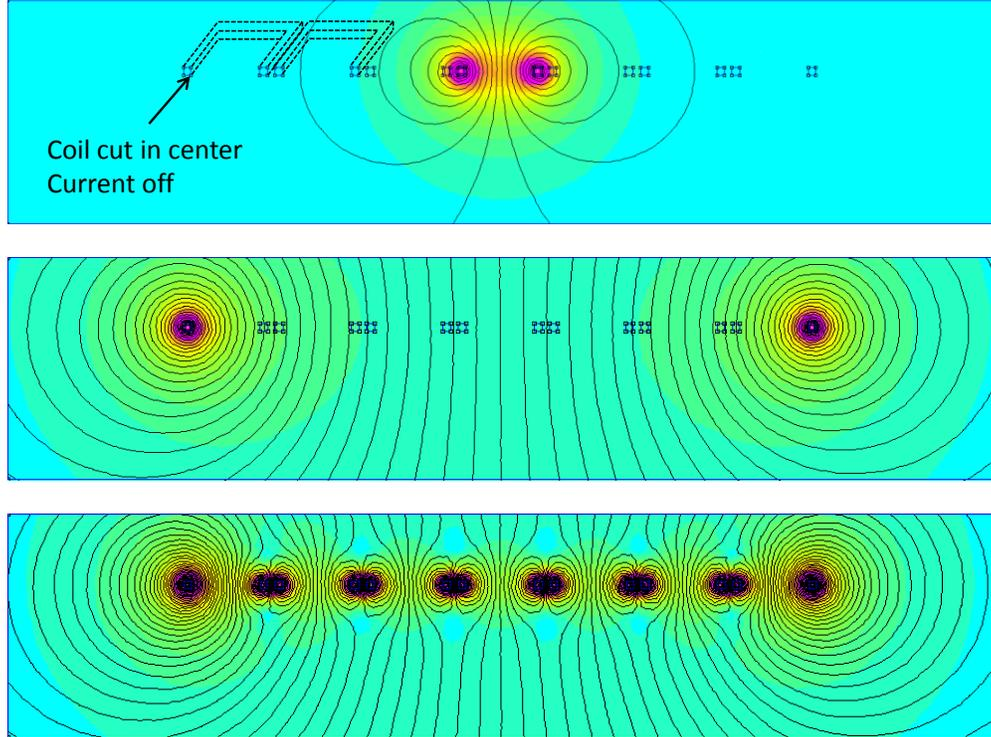
**Figure 3: 2D modeled fields for a small, a large size coil and an array of coils**
