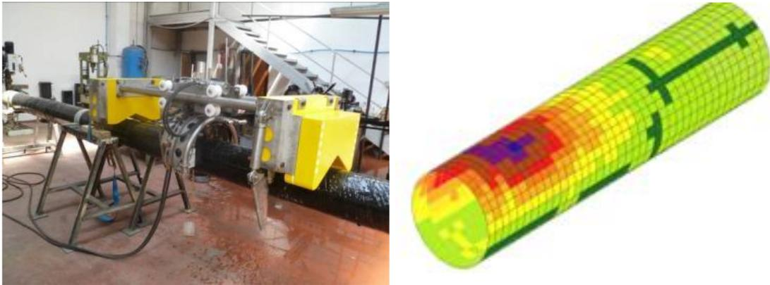
**Figure 1: Left Subsea inspection device for PEC. Right: depiction of inspection results (by Impresub [4])**
