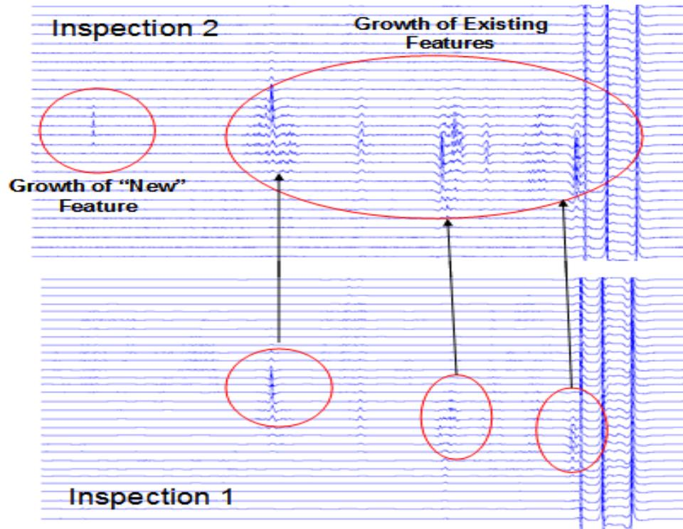
Figure 3: Detailed Corrosion Growth Assessment
