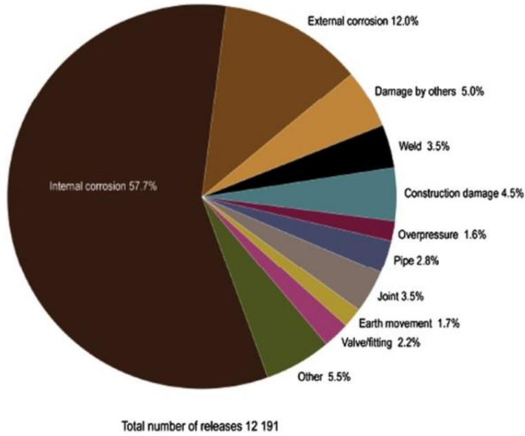
Figure 1. Pipeline main cause of failures, Canada, Alberta (1980-2005).
