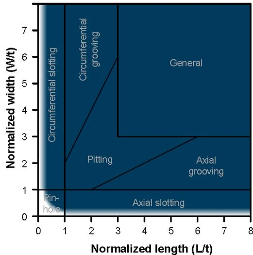
**Figure 5: POF feature classification diagram. Colored area indicates application range of EVO Series 1.0 UM tools for detection, classification, and sizing with  $t = \text{minimum \{Wall thickness, 10mm\}}$ .**
