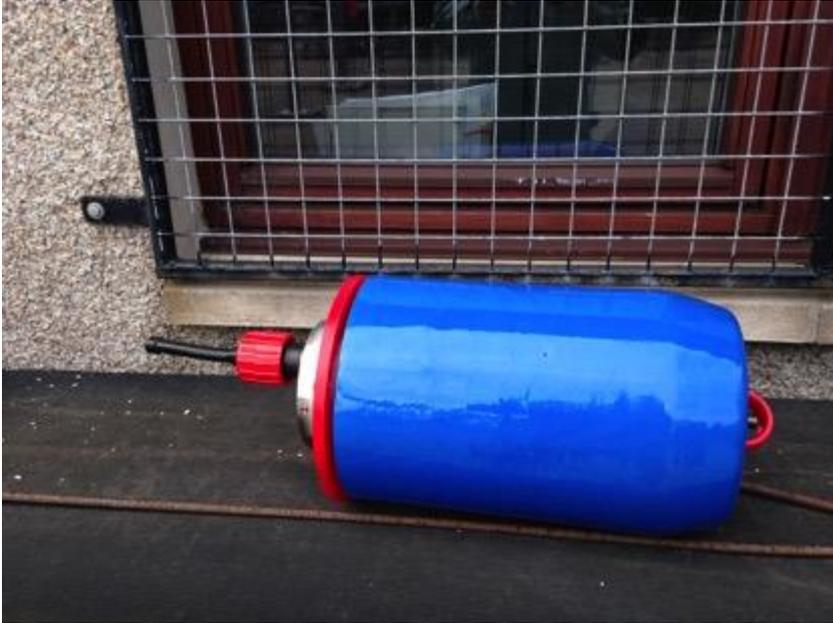
**Figure 4: 2<sup>nd</sup> generation foam pig with PU disk bolted to the rear flange of the internal pressure vessel.**
