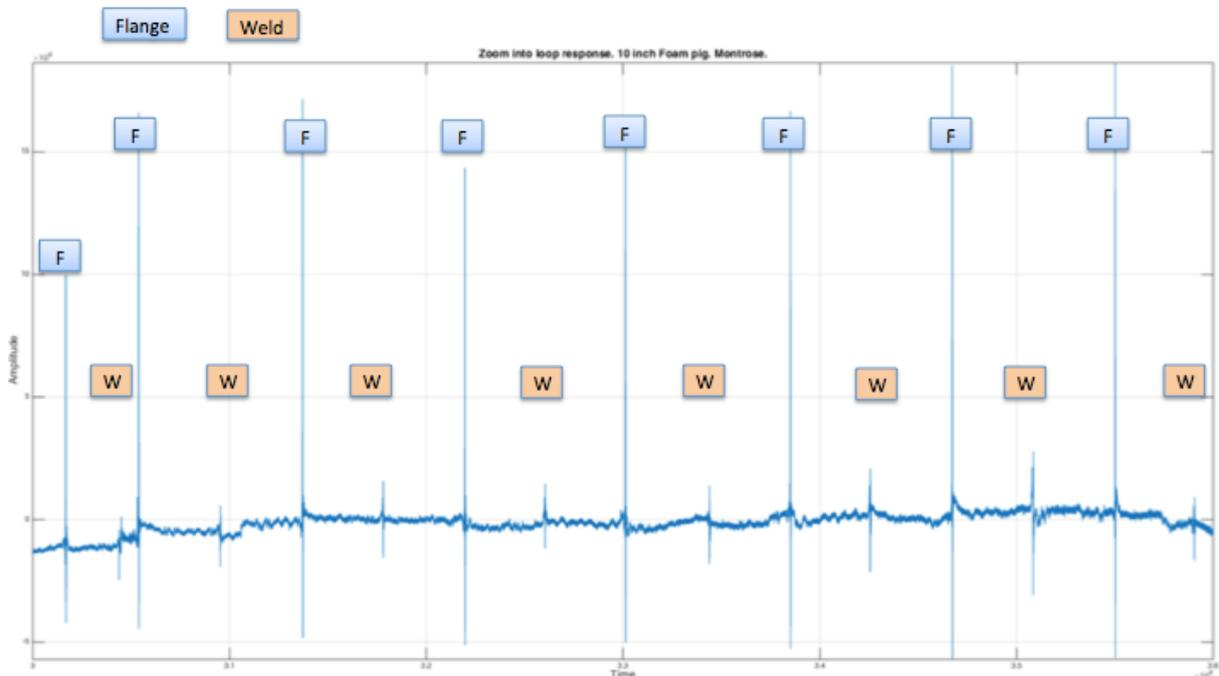
**Figure 10: Shows the uniform signals along the straight sections of the pipeline**
