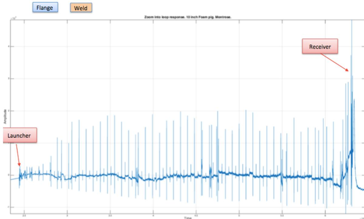
**Figure 8: 1 km of data from the Montrose test loop**
