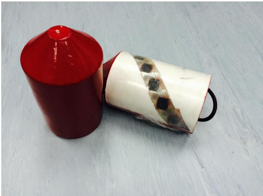
**Image 2: 1<sup>st</sup> Generation foam pig. Sensors arranged in helical array. No PU cup was included in the design at this stage.**
