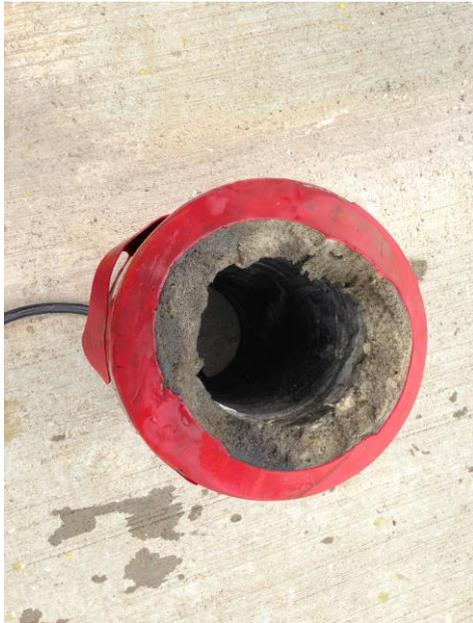
**Image 3: Failures occurred when the internal pressure vessel blew through the nose of the foam. The foam body alone is not strong enough to hold the pressure vessel in place. This is especially the case for smaller diameter tools.**
