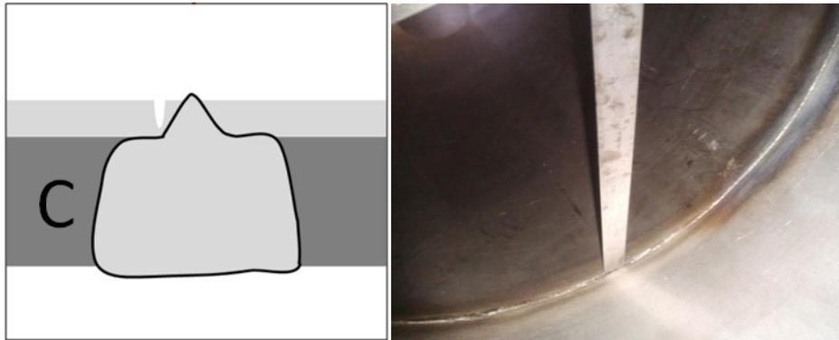
**Figure 4: Crack-like defects in the CRA-weld**
