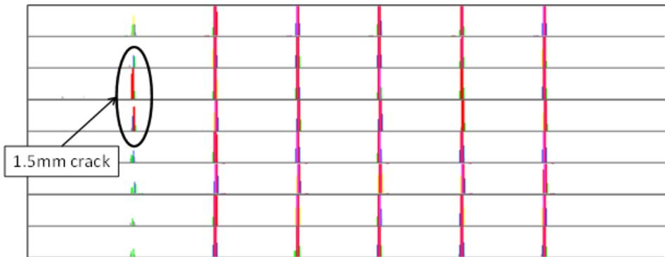
**Figure 12: Signals from the cracks obtained from the Multi-Differential Sensor**
