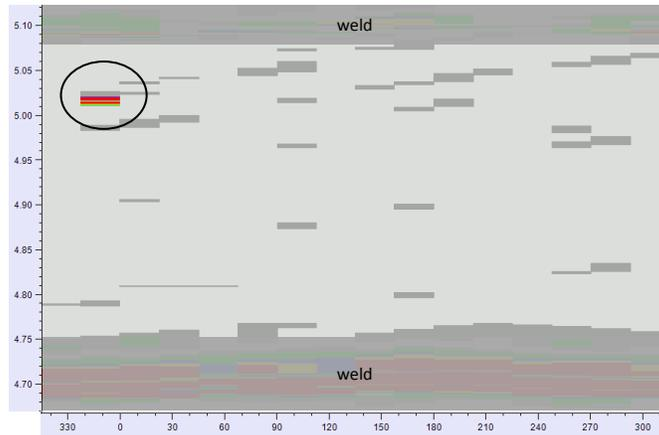
**Figure 11: Signal of a base material crack-like defect.**
