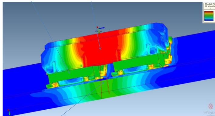
**Figure 6: Magnetostatic modeling of the magnet unit.**
