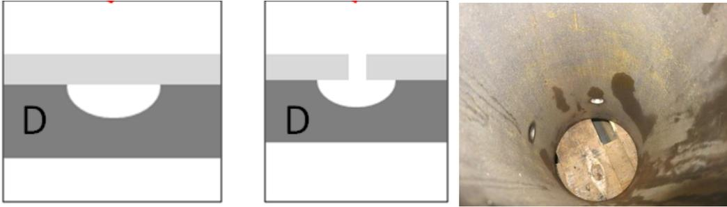
**Figure 5: Crevice Corrosion Defect Type**
