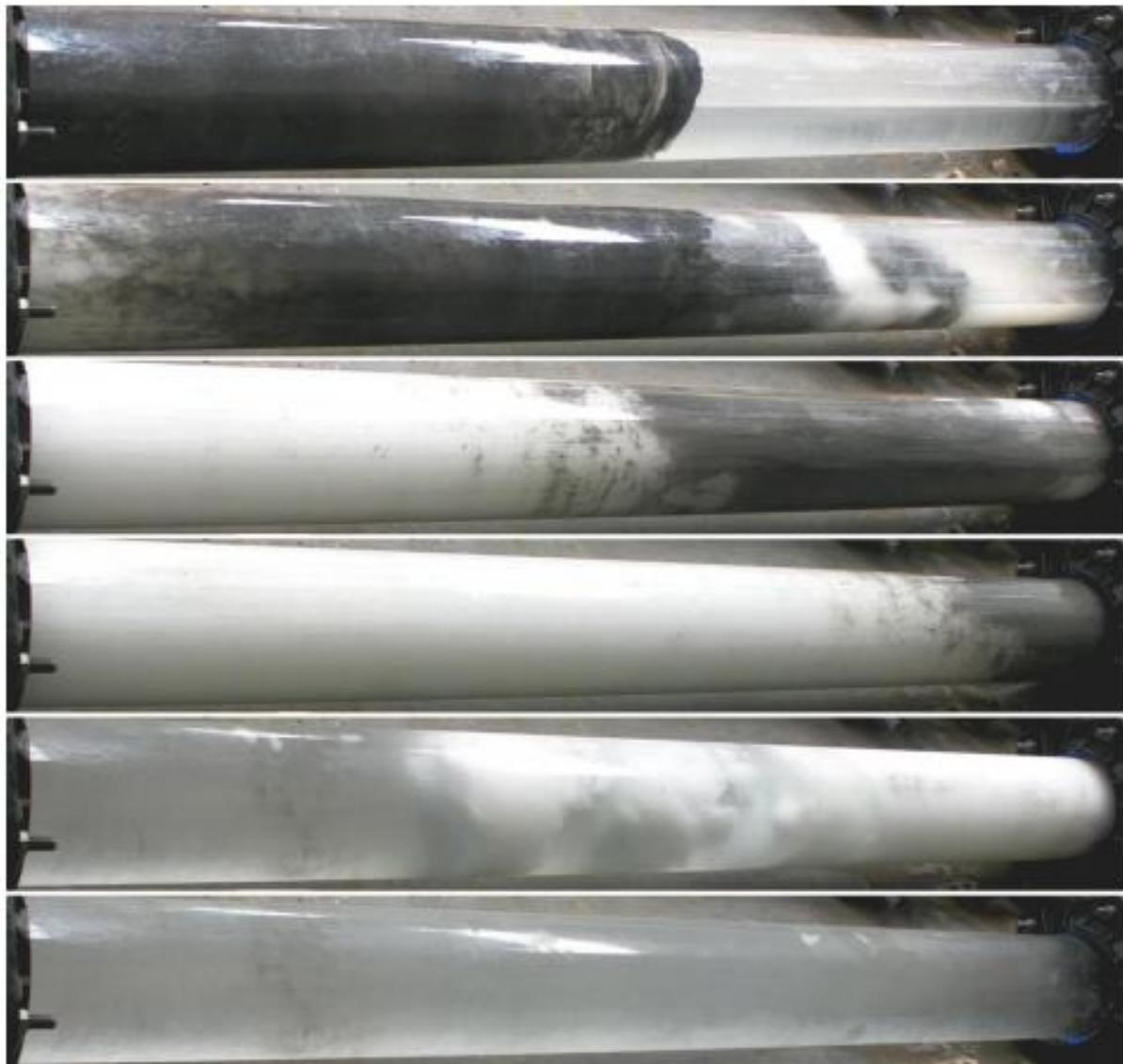
Figure 2 Flowing from left to right: an ice pig removes soft petroleum wax smeared in an 8" clear pipe.
