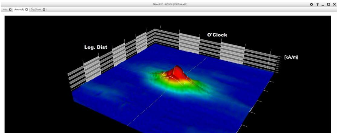
Figure 1. Example of 3D MFL-A Ultra data visualization
