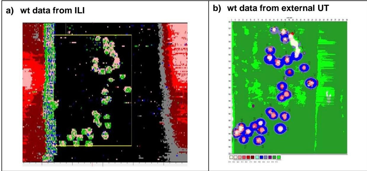
**Figure 8:** Ultrasonic C-scans (WT data) showing disbonded spots in clad pipe.
