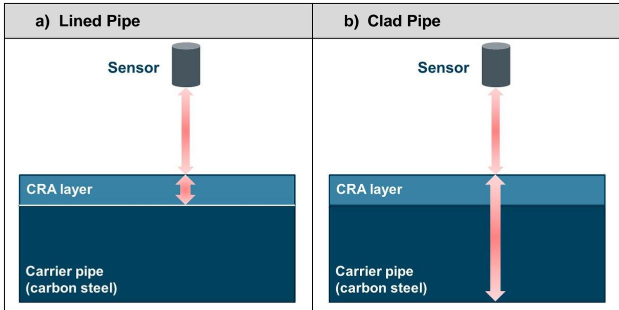
Figure 5: Ultrasonic propagation in lined pipe (a) and clad pipe (b)
