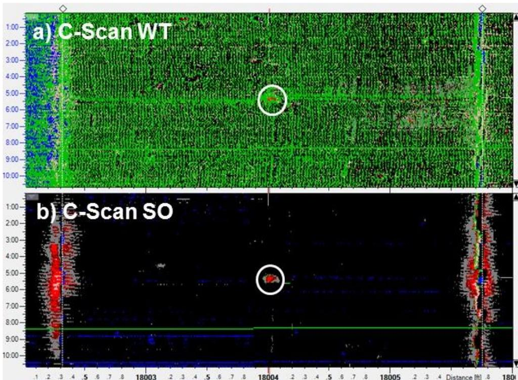
**Figure 7:** Ultrasonic C-scans as recorded in CRA pipe (clad pipe, weld overlay) showing an internal pit: a) wall thickness data b) standoff data
