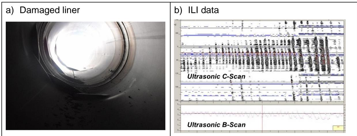
**Figure 9:** Damaged liner in lined pipe (a) and corresponding ultrasonic ILI data (b)
