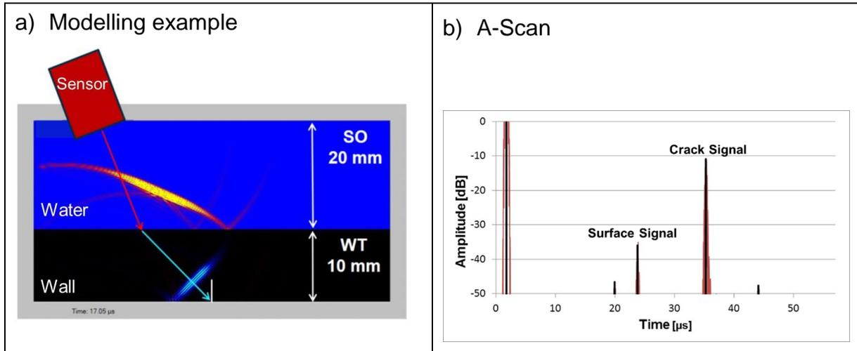
**Figure 10:** Ultrasonic crack inspection using 45°- shear waves in the pipe wall
