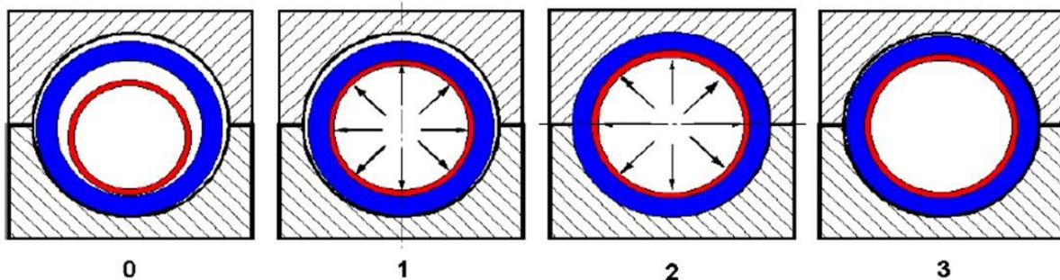
**Figure 2:** Manufacturing of lined CRA pipe by hydraulic expansion [2]
