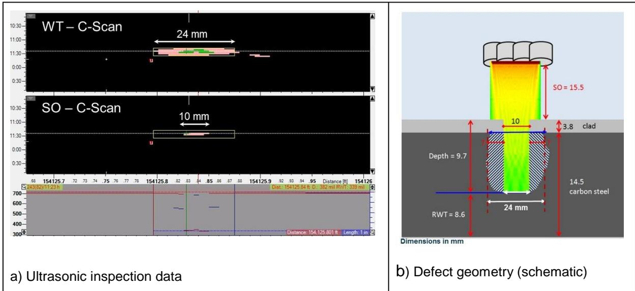
**Figure 6:** Through-clad pinhole extending into the CS carrier in roll-bonded clad pipe
