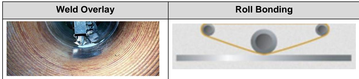
**Figure 2:** Common manufacturing methods for clad pipe
