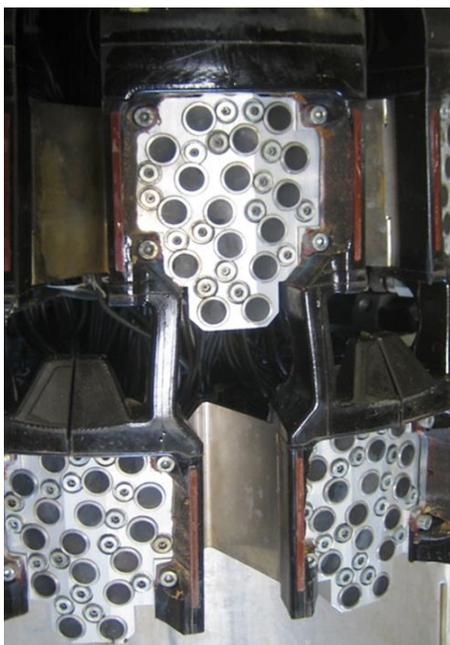
**Figure 4:** Example of sensor carrier for high resolution ultrasonic metal loss inspection (UMp for pitting resolution) with 4 mm circumferential sensor spacing
