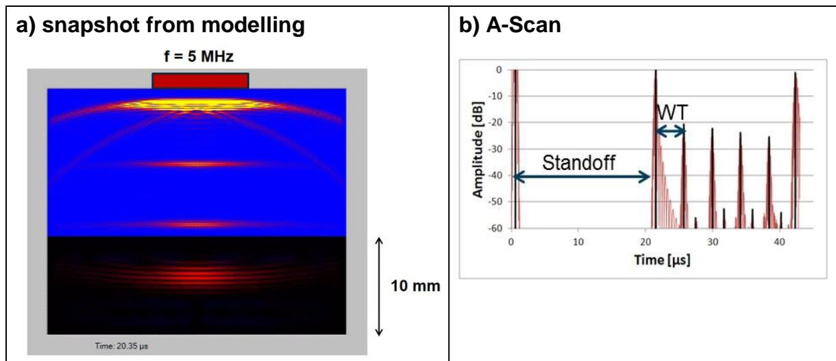
**Figure 3:** Principle of ultrasonic wall thickness measurement using longitudinal waves with straight incidence (a: modelling example; b: resulting A-scan)
