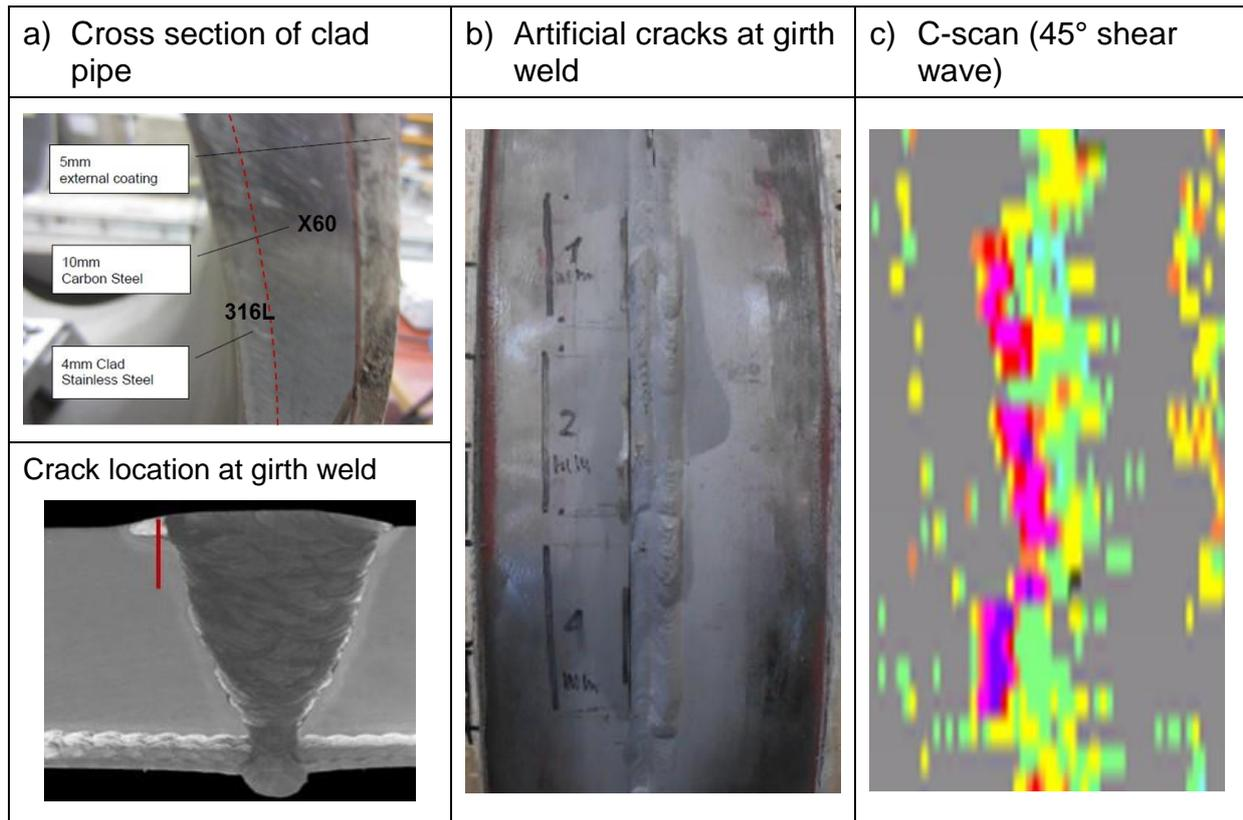
**Figure 11:** UT results from in-line crack inspection of a girth weld in clad pipe
